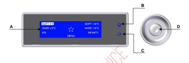
**A–Display**: Displays all the information relative to the menus on the board and the application in progress.
