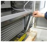
Remove the electrical panel locking screw.
